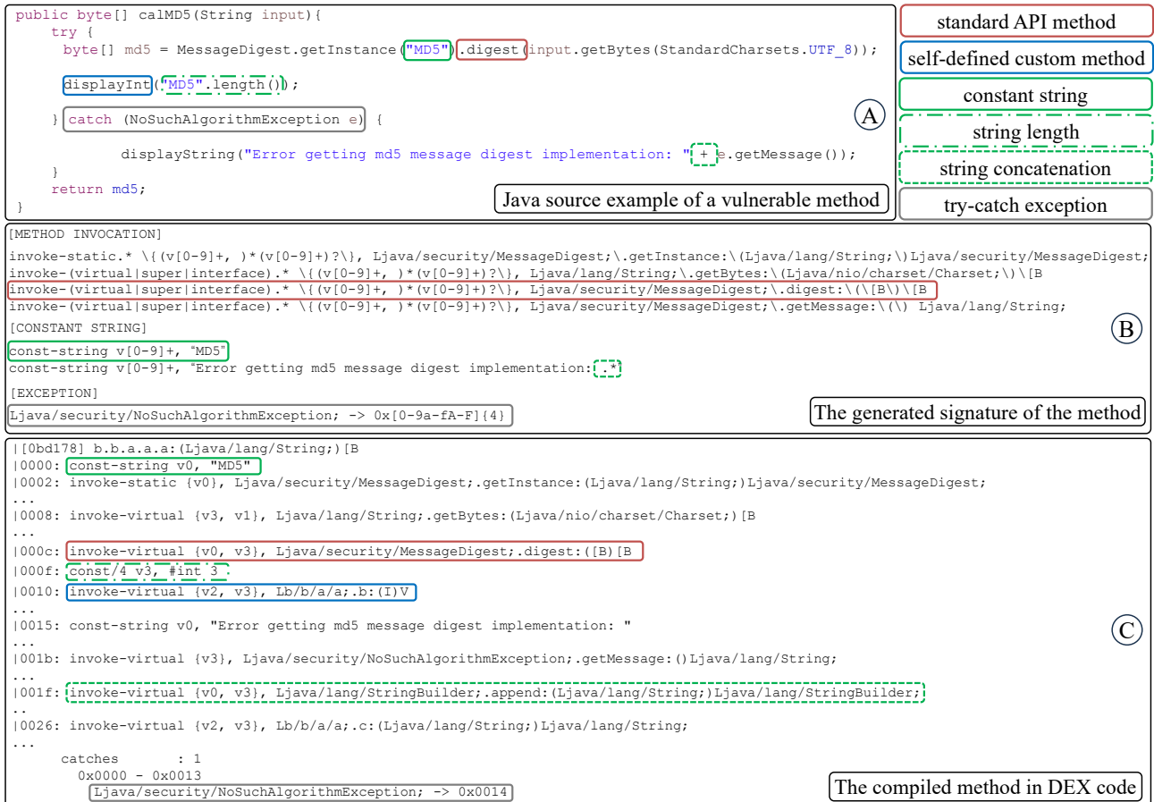
Figure 3: An example of the Java source, the generated method signature, and the matched DEX code. For simplicity, some unimportant instructions are omitted. The legends in the top right corner explain the meanings of different boxes.
