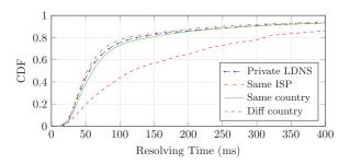
Figure 4: CDF plot of DNS resolution time for different DNS deployments. The time includes both network delay and server response time (e.g., its recursive querying time).
