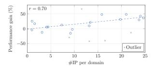
Figure 8: Relationship between performance gain by using IP anycast and the number of IP per domain. Each point is an SLD. Outliers are identified by robust regression. *r* stands for the Pearson correlation coefficient.
