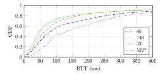
Figure 3: CDF plot of median RTT for different ports. "522\*" includes 5222, 5223, and 5224.
